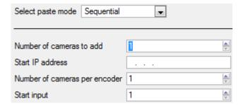
**Start IP Address** will determine the IP address of the first new camera being added. The IP addresses will be incremented from here. (So, make sure no IP addresses in this range have been used.)
